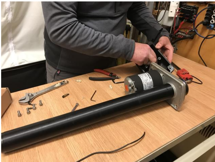
Fixing the Raymarine autopilot drive unit
