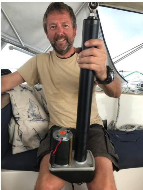
Dismantling the autopilot drive unit
